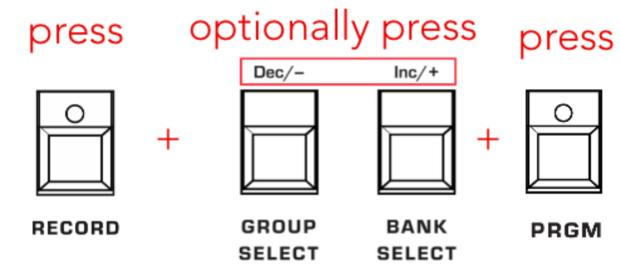
Be careful when RECORD is enabled. You can change GROUPS and BANKS without executing WRITE, but once you press a PROGRAM SELECTOR button (1-8) for the "ones" digit, the RECORD command is executed and the program at that location is overwritten.
